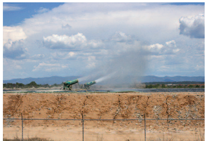
Water cannons are used to increase evaporation of fracking fluid at some plants, contributing to air pollution. © tedx
